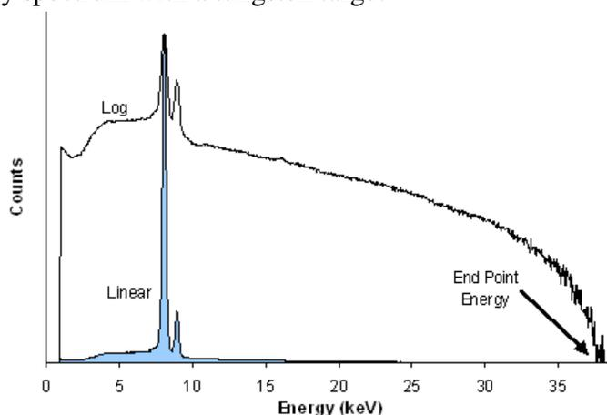
Figure 8. COOL-X x-ray spectrum with a copper target
