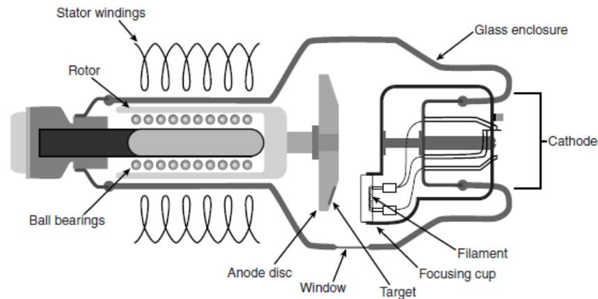
Figure 2. Diagram of an X-ray Tube
