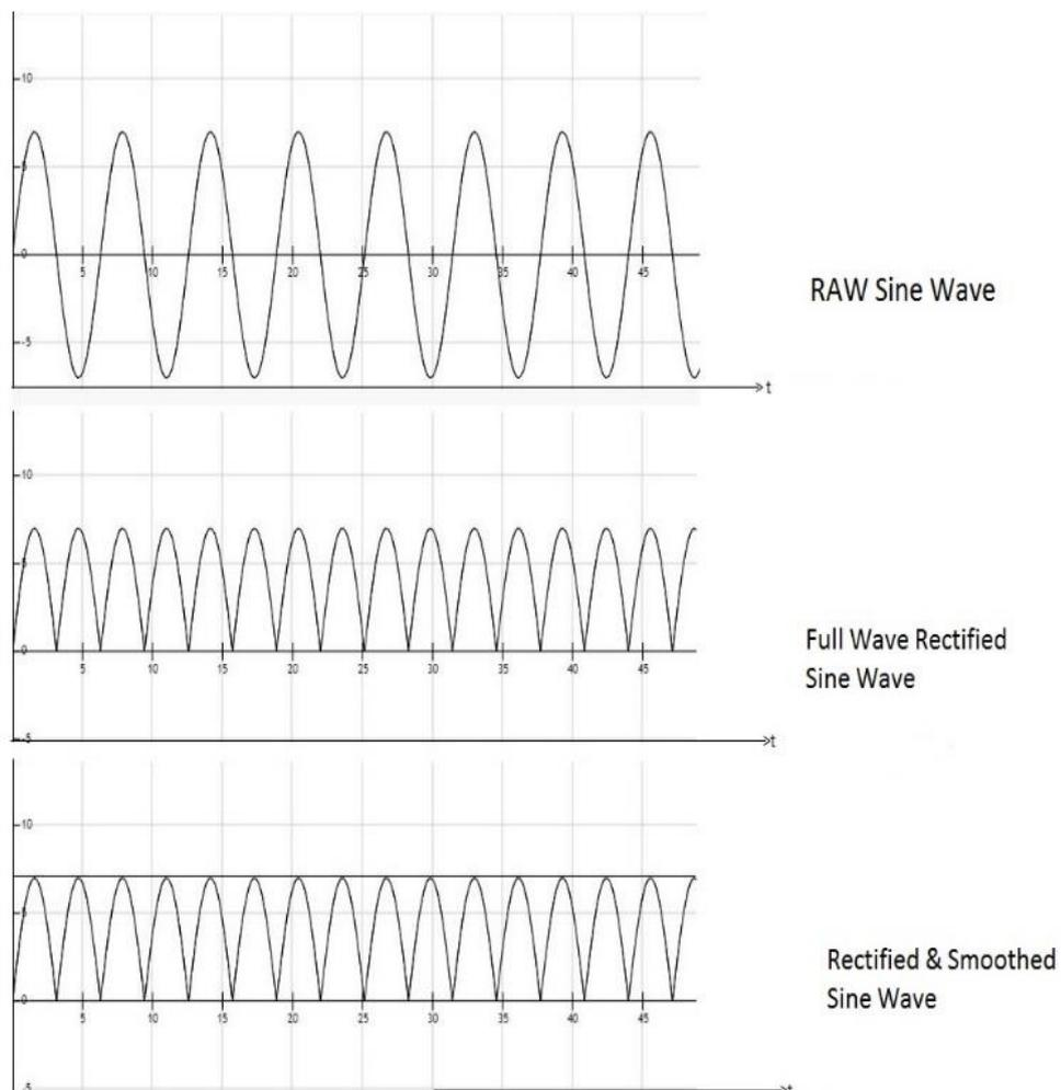
Figure 1. Full-wave rectification of a sinusoid.
