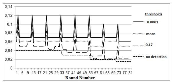
**Figure 7.** Total energy consumption on a 50 node system for detecting the sinkhole attack for different values of thresholds, including 0.0001, average amount of energy consumed in the previous round and 0.17. The results compared with a system without any detection mechanism.
