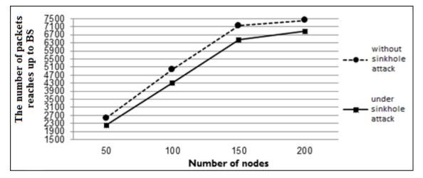
**Figure 5**. The number of packets arrived at BS when the system is under sinkhole attack and is in safe mode for a 50,100,150 and 200 numbers of nodes.
