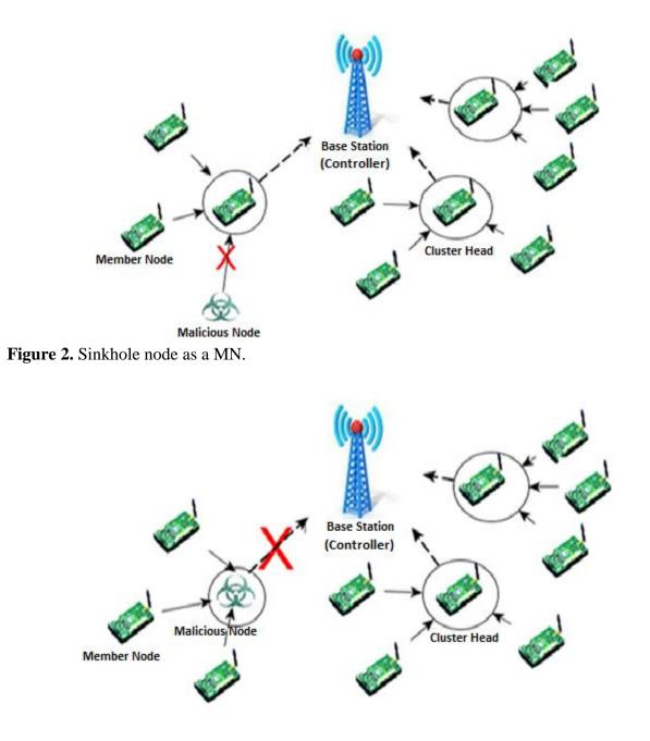
Figure 3. Sinkhole node as a CH.
