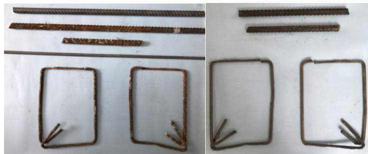
Figure 4. View of reinforcements after accelerated corrosion test.
