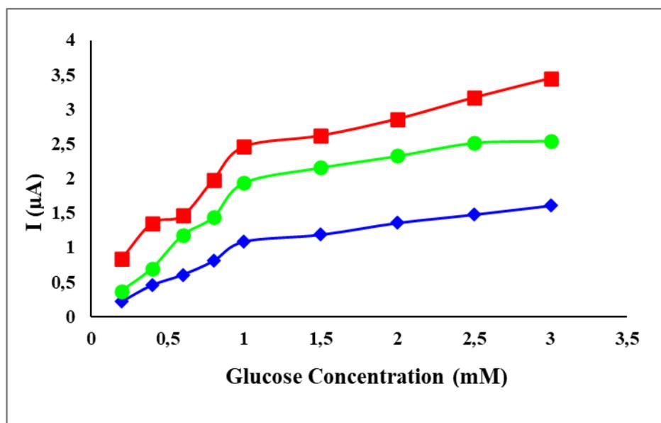
**Figure 2.** Current responses obtained for glucose concentration of Pt/POT-GOD electrodes fabricated by POT film synthesized for different scan rates; ( $\blacklozenge$ : 20 mV/s-2 segment,  $\blacksquare$ : 50 mV/s-4 segment,  $\bullet$ : 100 mV/s-8 segment).
