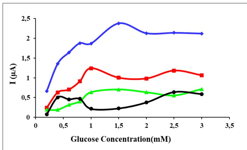
**Figure 1.** Current responses obtained for glucose concentration of Pt/POT-GOD electrodes fabricated by POT film synthesized for different concentrations of o-toluidine such as 40 mM (♦); 50 mM (■); 60 mM (▲) and 70 mM (●).
