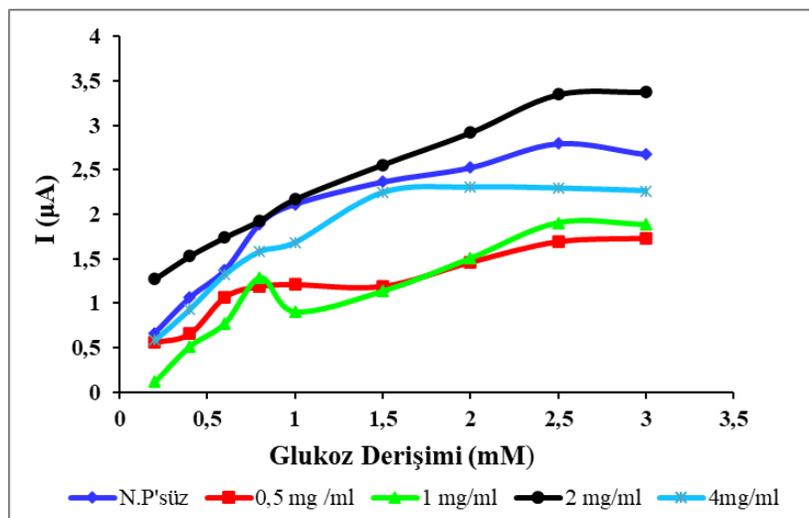
**Figure 5.** Current response of POT based biosensors modified with ZnFe<sub>2</sub>O<sub>4</sub>NP. —♦—: ZnFe<sub>2</sub>O<sub>4</sub>NP-free; —■—: 0,5; —▲—: 1,0; —●—: 2,0 and —\*—: 4,0 mg/ml.
