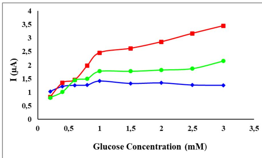
**Figure 3.** Current responses obtained for glucose concentration of Pt/POT-GOD electrodes fabricated by POT film synthesized for different segments ( $\blacklozenge$ : 2 segments,  $\blacksquare$ :4 segment,  $\bullet$ :6 segment).
