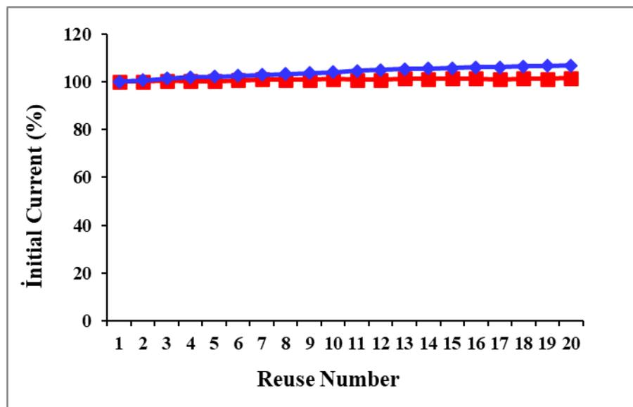
**Figure 6.** Operational stabilities of Pt/POT/Chi-GOD and Pt/POT/Chi-GOD-ZnFe<sub>2</sub>O<sub>4</sub>NP electrodes.
