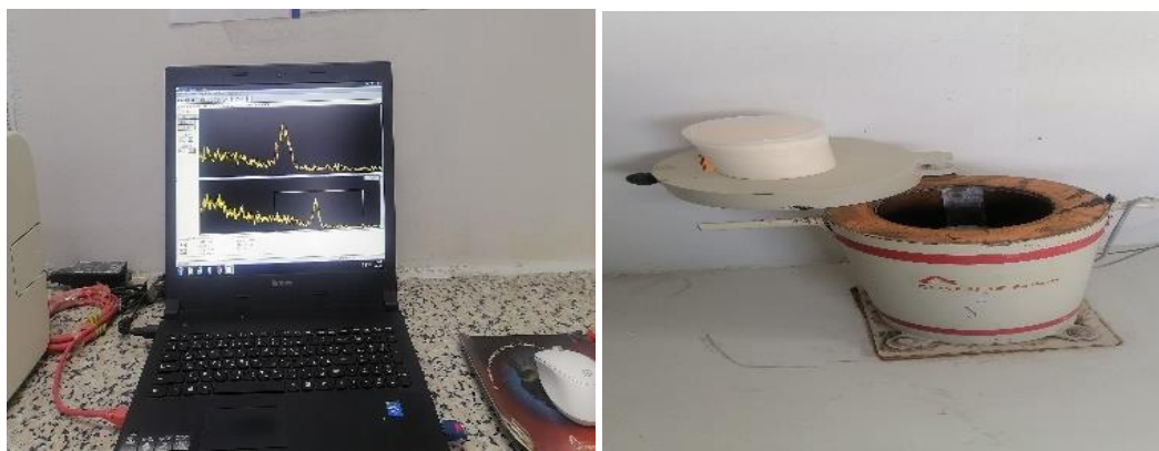
Figure 1. NaI (TI) detector and the data acquisition system (State Company for Foodstuffs Trading laboratory)
