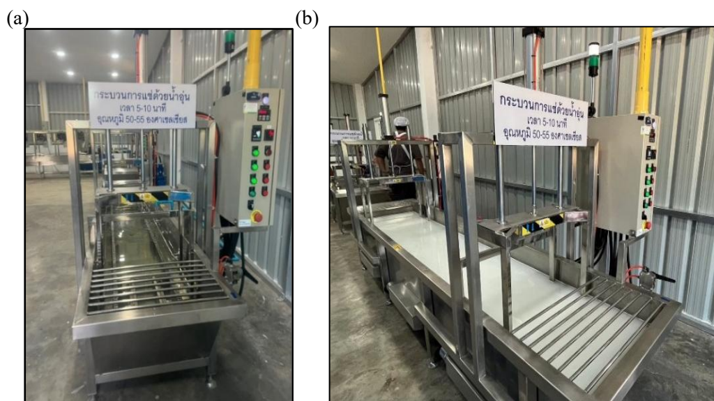
Figure 2. (a) Front view and (b) side view of the hot water treatment machinery integrated into the postharvest production line.
