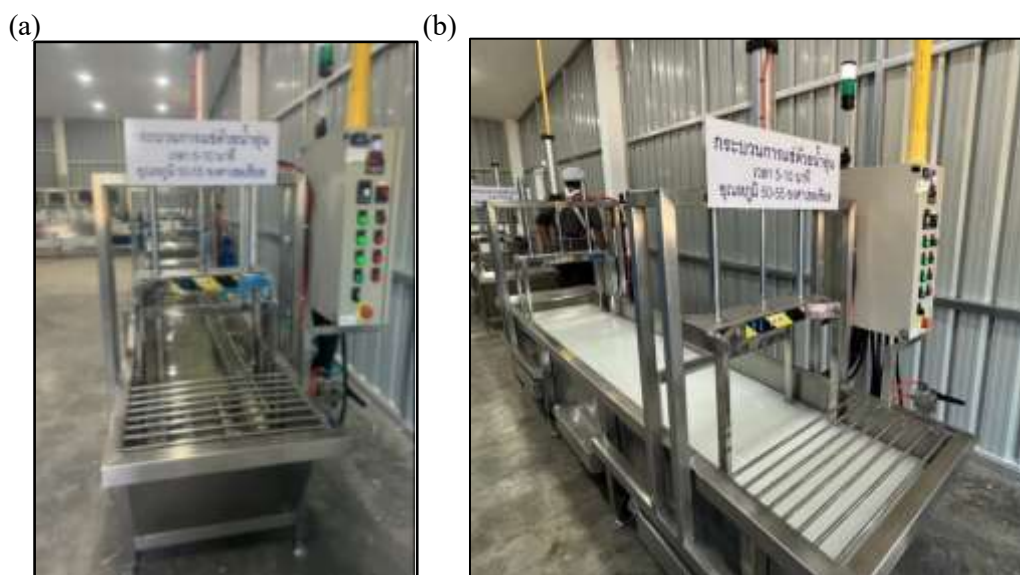
Figure 2. (a) Front view and (b) side view of the hot water treatment machinery integrated into the postharvest production line.
