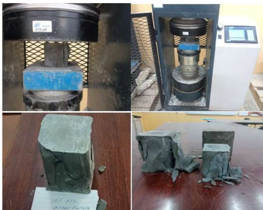
Figure 1 : some concrete specimens (PRPC) during and after test
