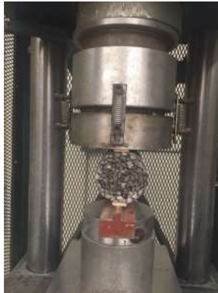
Fig. (4) Splitting tensile strength test of (100X200) mm porous concrete cylinder
