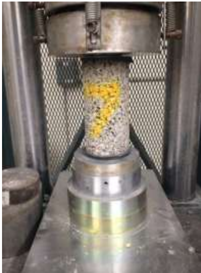
Fig. (2) Compressive strength test on (100 X 200) mm sulfur-capped cylinder
