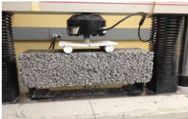
Fig. (3) Porous Concrete Beam Test Set-Up (150 × 150 × 450) mm
