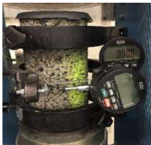
Fig. (5) Elastic modulus test of (100X200) mm sulfur-capped porous concrete cylinder
