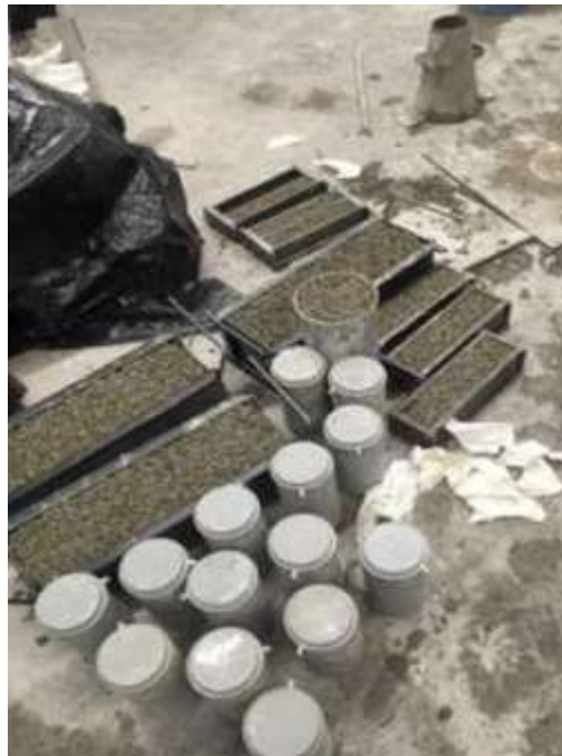
Fig. (1) Various types of specimens after casting
